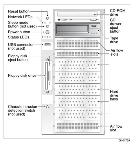
The table below describes the parts that are identified in the preceding diagram:
